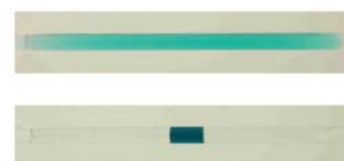
Loading of 1 \mu L dye sample into 10 \mu L microcoil NMR flowcell by segmented flow (bottom) avoids dilution seen in flow injection (top).
